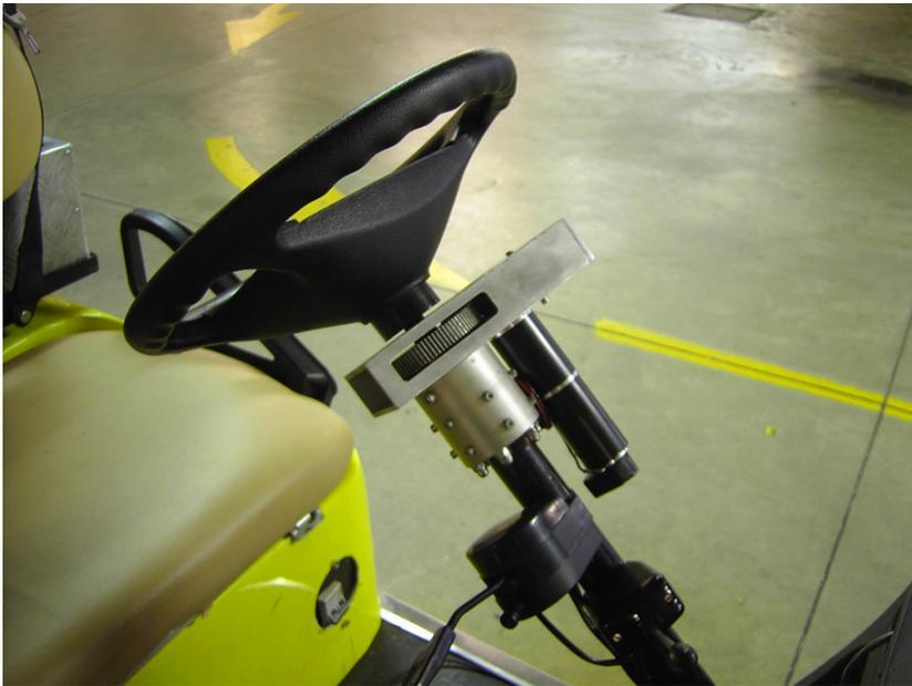
Figure 6.10: The final, fully operational robotized steering system. The steering wheel is plugged on top of the steering column, allowing humans to operate the steering system.
