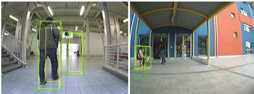
Figure 4.7: Some mistakes of the detection system: (left) a false positive; (right) a false negative, notice that the person detected is seating, a situation missing from the training set.
