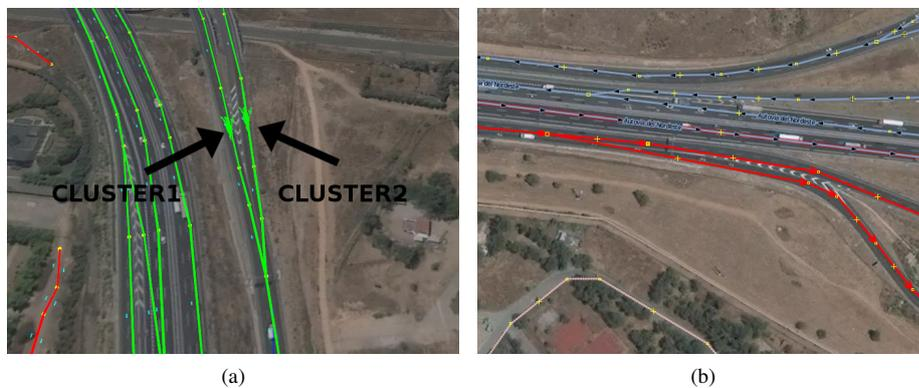
Figure 5.31: The figure depicts a typical Y-junction. Since the ramp follows the route of main road, there is no chance for the OpenStreetMap component to distinguish between the two clusters.
