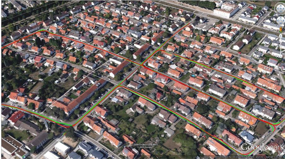
Figure 3.1: Example result using the proposed framework on run 2011\_09\_30\_drive\_0018 of the KITTI dataset, and the corresponding OpenStreet-Map road network. The red path is the GPS-RTK and plays the role of ground truth. In green, the localization results of our framework.
