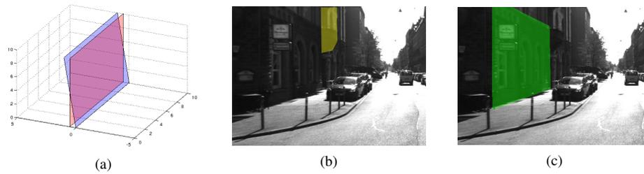
Figure 3.12: Perpendicularity correction. In Figure 3.12a blue color represents the original plane and red the plane made orthogonal to the ground plane. Figures 3.12b and 3.12c depict a typical façade with a balcony, which introduces a bias in the plane estimation using our pure geometric approach.
