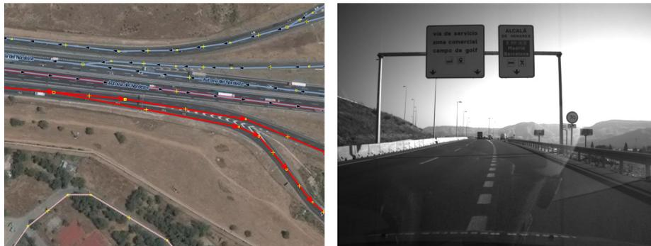
Figure 3.17: The figure depicts a common highway scenario with two parallel roads. In these cases, a simple map matching algorithm is not able to discriminate the correct vehicle position.
