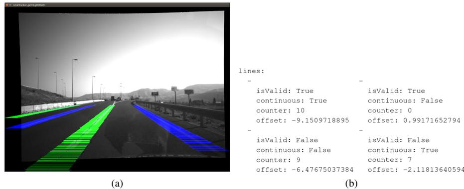
Figure 3.18: In the figure, the detected lines are re-projected in the 3D image-space. The corresponding line measurements are depicted on right.
