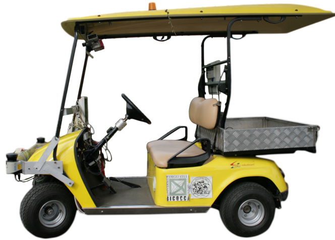
Fig. 17. Our vehicle at the current development stage. On the front the three LIDARs can be noticed.
