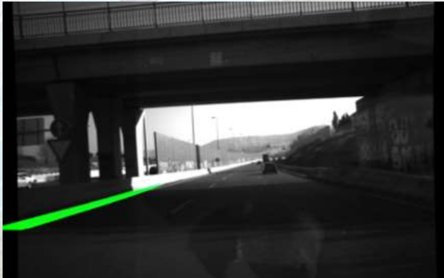
Only leftmost line detected due to illumination issues
