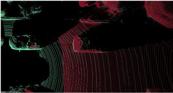
Fig. 6. Misalignment between LIDAR and camera-based PCs. The camera-based PC has been computed using the colour camera images and the projection parameters obtained for the black-and-white cameras, while the other PC is from the LIDAR. The two has been superimposed using the poses of the two sensors (the stereo rig and the LIDAR) w.r.t. the vehicle. Here the misalignment is less than 0.2m.
