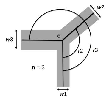
Fig. 1. The intersection model used to generate the intersections: c represents the intersection center, n the number of road segments,  $w_i$  and  $r_i$  the width and the orientation w.r.t. the road segment where the vehicle is.
