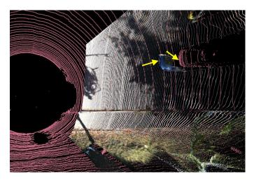
Fig. 5. Misalignment between LIDAR and camera-based PCs. The camera-based PC has been computed using the colour camera images and the projection parameters obtained for the colour cameras, while the other PC is from the LIDAR. The two has been superimposed using the poses of the two sensors (the stereo rig and the LIDAR) w.r.t. the vehicle. At the car bumper the misalignment is just more than 1.9m.
