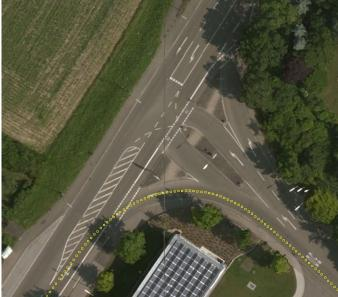
Fig. 4. The figure depicts intersections that cannot be represented using the model proposed in Figure 1: multiple laterally displaced arms plus traffic island or other raised areas; the yellow dotted line does not carry any particular meaning, please just dis-regard it.
