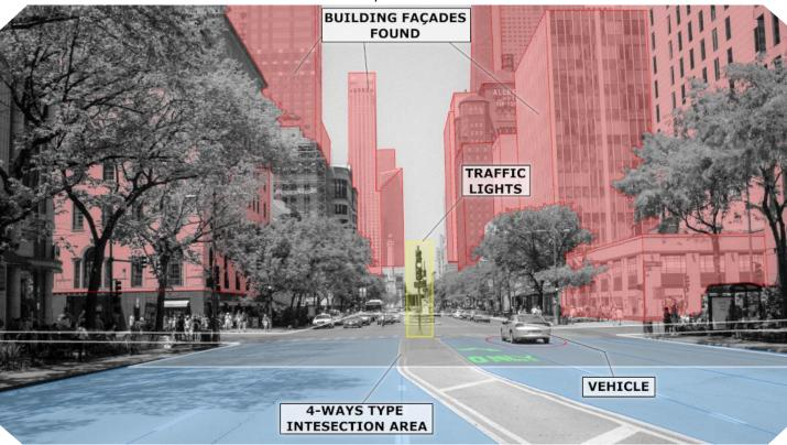
Automated vehicle navigation in GPS-denied-or-limited areas may benefit from the detection of specific urban features, such as intersections, road typologies, multi-lane detection, traffic-flow detection without road markings, traffic understanding and modeling, building detections, cartographic maps exploitation, cartographic maps augmentation and other features that we are eager to see used for the localization purposes.
